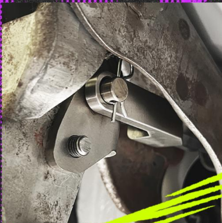
Stainless Steel Push Rod, Bolt-On 6:1 Pedal Adapter, Stainless Steel Clevis & Hardware
